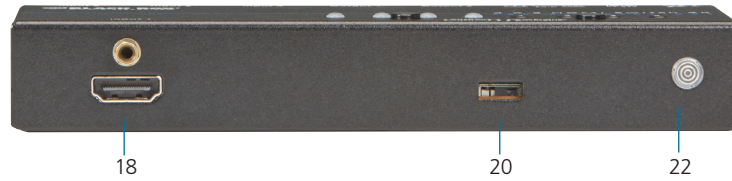
Figure 2-4. VSW-HDMI4X2-4K front panel.
