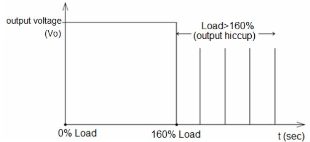
Additionally, if the 24 Volts' out is  $>100\%$ ; but  $<160\%$  for a prolonged period of time (depending on the load), the Over Temperature Protection (OTP) will be activated due to high temperature on critical components. The power supply will then go into latch mode.
